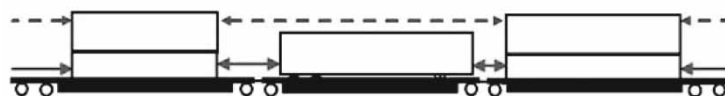
Fig. 8 Illustration of upper level gaps (dashed lines) and lower level gaps (solid lines)
