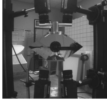
Fig. 6. The implementation of a six-sided DMP camera prototype.
