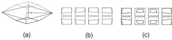
Fig. 5. Maximizing sensor utilization and enforcing the uniform resolution constraint. (a) Mirror pyramid and viewpoint. (b) Ensuring maximum sensor utilization by using the maximum possible focal length or the minimal possible FOV to image the entire mirror face associated with each camera. Different cameras capture images at different resolutions. (c) Enforcing uniform resolution by using a constant FOV for all cameras and, thus, reducing overall sensor utilization.
