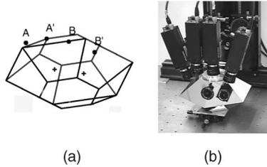
Fig. 8. (a) A design showing a 6-face pyramid and only two pairs of cameras ( $AA'$ ,  $BB'$ ). Each pair is associated with one face and the two viewpoints are shown as crosses (+). (b) The experimental setup implementing the design in (a). Note that the left virtual camera (inside the pyramid) is a combination of the mirror images of two cameras from two adjacent mirror faces.
