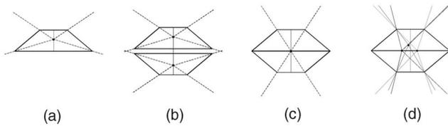
Fig. 1. The evolution of mirror pyramid cameras. (a) Original design by Nalwa [4]. (b) Stereo design by Kawanishi [28], vertically stacking two of the cameras from (a). (c) Double vertical FOV design by Hua and Ahuja [29]. (d) Generalized multiview design, shown with three viewpoints [2], [3], [30]. In general, the design is able to accommodate an arbitrary number of viewpoints placed in arbitrary configurations.
