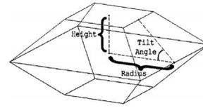
Fig. 2. The geometry of a mirror pyramid.
