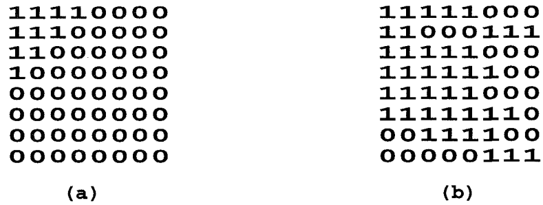
Figure 1: Projection operators for the proposed method on an 8x8 image block: (a) put all coefficients with mask value zero to zero in the DCT domain. (b) constrain the values of the pixels with mask value 1 to the actual DFD values in the spatial domain.
