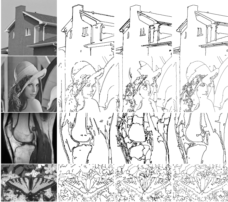
Fig. 7. Segmentation results. First column: input image, second column: output of graph-based method, third column: output of mean-shift based method, fourth column: our method. See text for details on input parameters.
