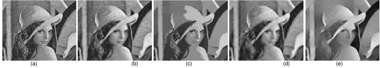
Fig. 5. Image Restoration Results Comparison Using Different Algorithms. (a) Noisy image; (b) Coherence enhancing diffusion; (c) Nonlinear diffusion; (d) Wavelet Denoising; (e) Reconstructed image using our gradient-based image restoration algorithm.
