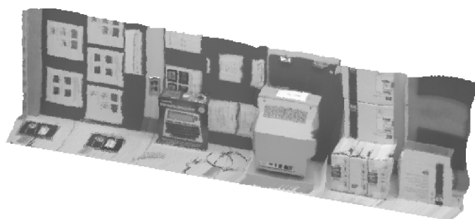
Fig. 13. Reconstructed 3D surface integrated from many partial views in the sequence, shown with original intensity viewed from an arbitrary direction.
