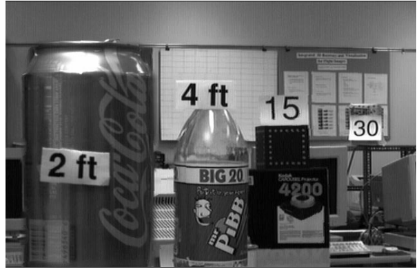
Figure 7: Image of scene taken with omni-focus camera.
