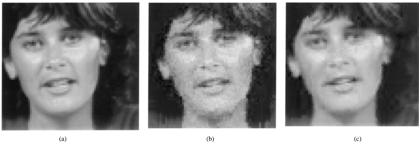
Fig. 7. Part of a frame from Miss America sequence ( \mathcal{M} = 4 ): (a) original, (b) block based approach, and (c) region based approach.
