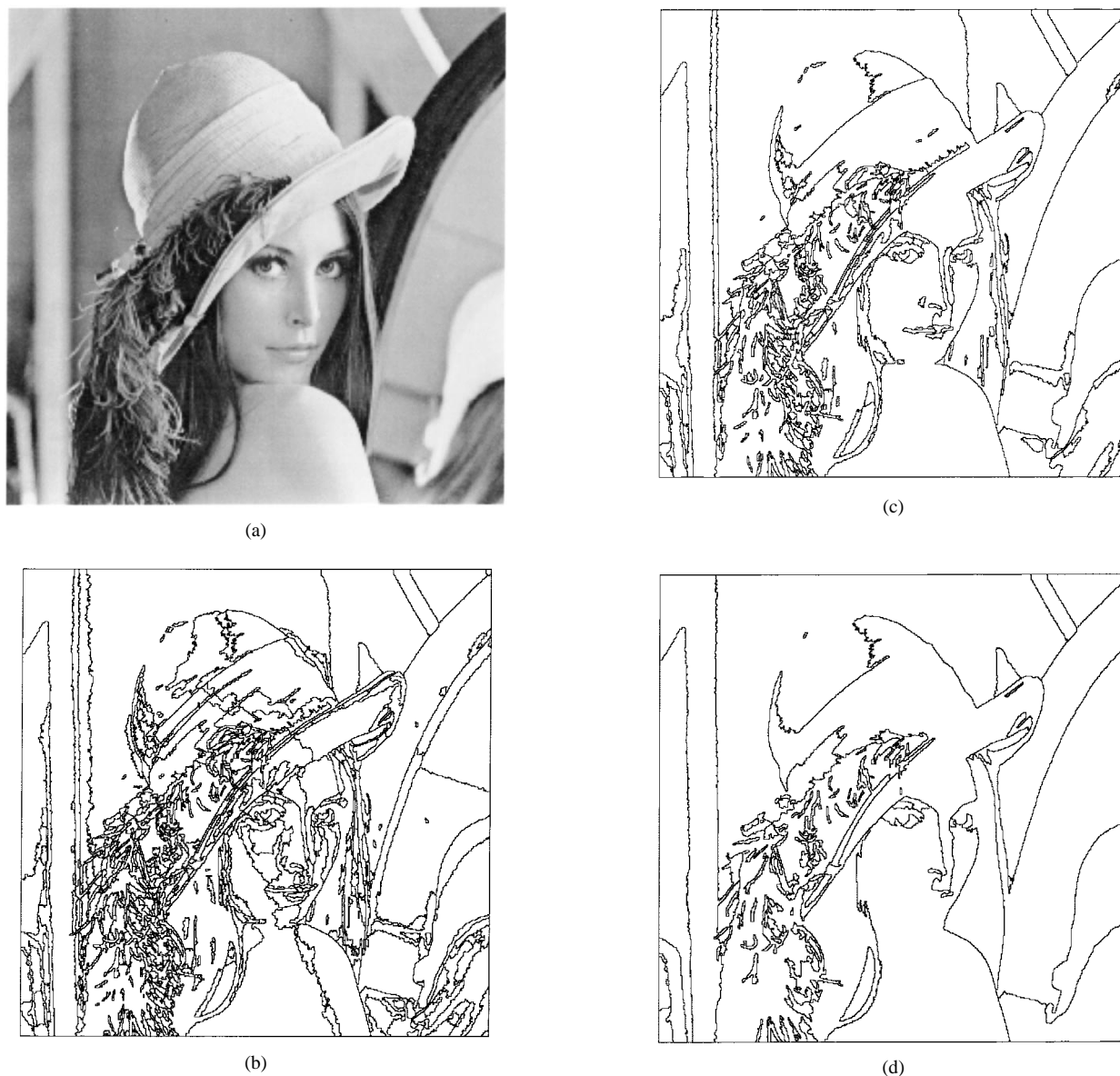
Fig. 2. (a) Actual image and (b) different scales of segmentation given by the multiscale segmentation algorithm. (c) and (d) Different scales of segmentation given by the multiscale segmentation algorithm.
