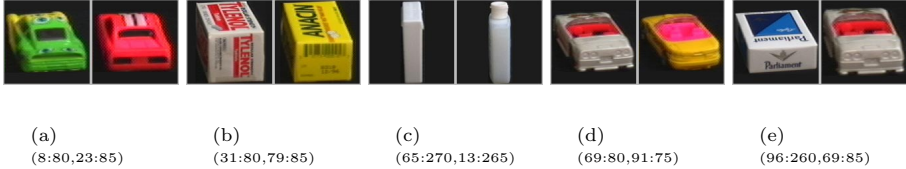
Fig. 6. Mismatched objects using the nearest neighbor method. (x : a, y : b) means that object x with view angle a is recognized as object y with view angle b . It shows some of the 54 errors (out of 3,600 test samples) made by the nearest neighbor classifier when there are 36 views per object in the training set.
