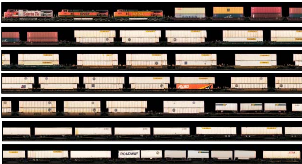
Figure 12. Example panoramic image of part of a train cut into multiple pieces for image display purposes
