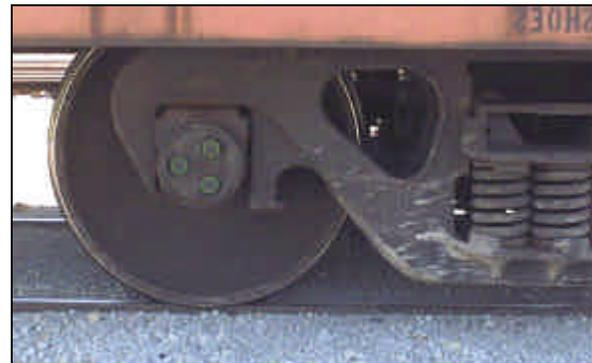
Figure 3. Bearing End Cap Bolts Identified
