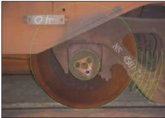
Figure 4. Missing Bolt Detection
