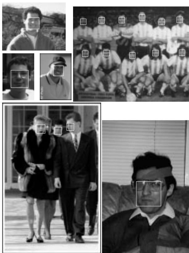
Figure 3. Sample experimental results using mixture of subspaces with Fisher Linear Discriminant on images from three test sets. Every detected face is shown with an enclosing window.
