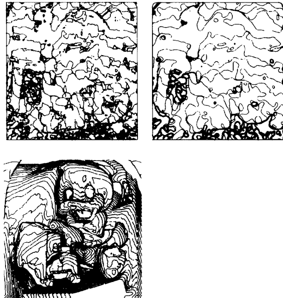
Figure 5: Level curves of the stereo result, level curves of the filtered stereo result and the level curves of the final surface.
