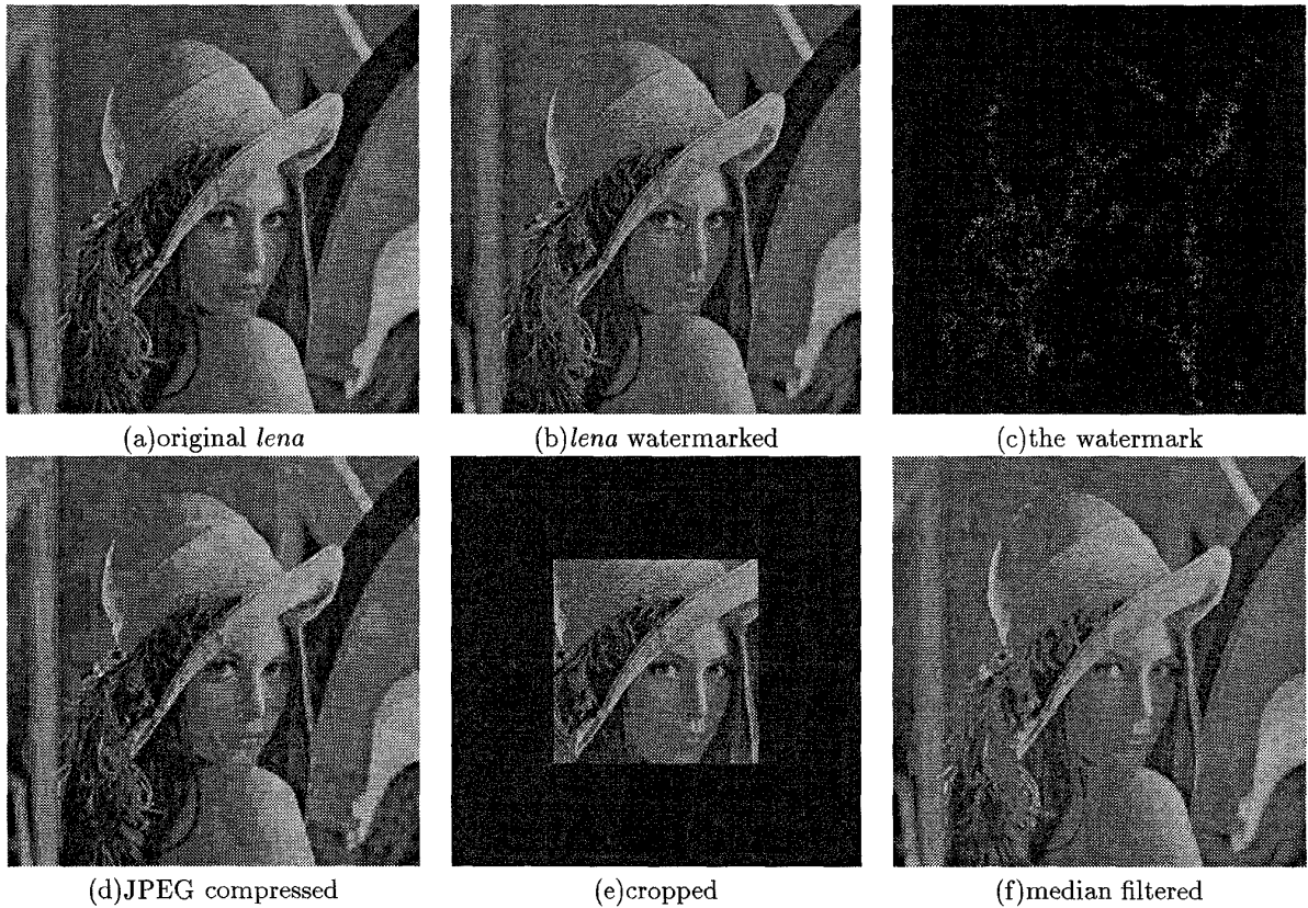
Figure 2: (a) original lena image (b) lena watermarked with our method (c) The difference of (a) and (b) i.e. the watermark as it appears in the spatial domain. Note that most of the watermark gets added in edge regions where it is perceptually not visible. The watermarked image in (b) and the difference image in (c) have been scaled for display purpose. Watermarked image in (b) with (d) JPEG 5% quality compression, (e) cropping to retain only the central portion and (f) median filtering with a 5 \times 5 window
