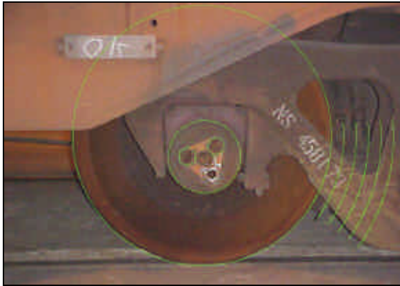
Figure 4. Missing Bolt Detection
