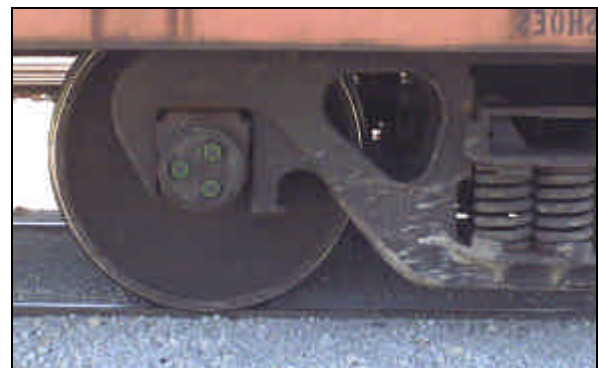
Figure 3. Bearing End Cap Bolts Identified
