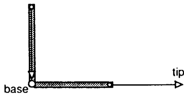
Figure 32. Singular configurations of a 2-link manipulator. The tip cannot move in the radial direction.
